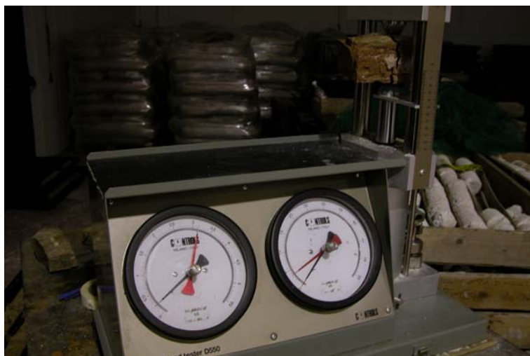
Figura 16 – POINT LOAD TEST
